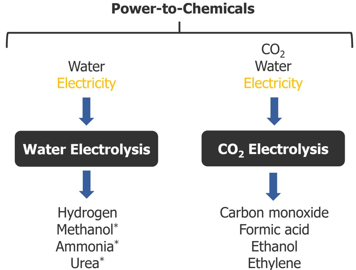
4 \*Methanol, ammonia, and urea are made from the hydrogen produced with water electrolysis
